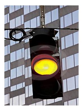
Based on the ITE formula, the length of the yellow interval increases with increasing approach speed. The formula also produces longer yellow intervals for approaches located on downgrades and shorter yellow intervals for approaches located on upgrades. For automobiles on a flat approach, the following yellow intervals are obtained from the ITE formula:
