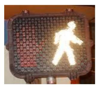
WALK intervals of greater than 7 seconds may be used where the duration of the associated vehicular green interval is long enough to accommodate it. The purpose of the WALK interval is to provide enough time for a group of waiting pedestrians to enter the crosswalk before the flashing DON'T WALK commences.
